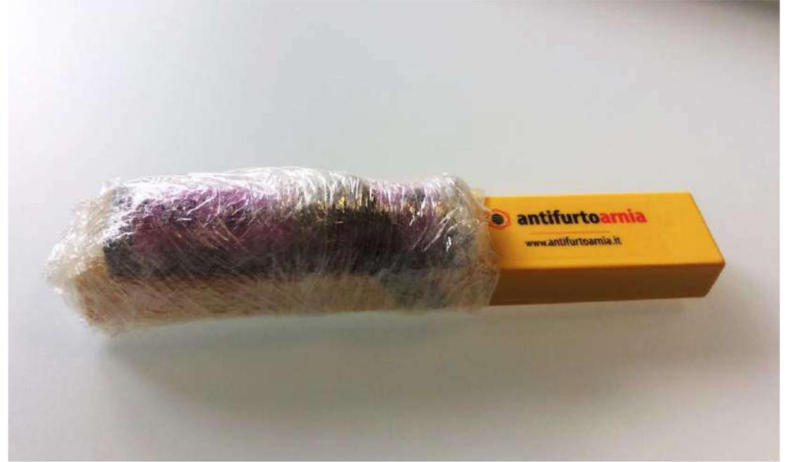
2. Wrap the part of the device containing the battery with a piece of plastic or film.
