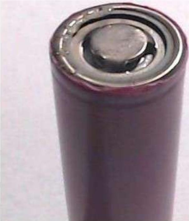
Damaged insulation – do not use
